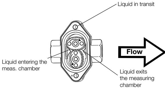
The positive displacement flow technology allows for precise flow measurement of most clean liquids regardless of the media conductivity. Other liquid properties also have a minimal effect on the performance of this type of meter. Flow profile conditioning is not required as with alternative flow technology options making oval gear installations simple to install in tight spaces and at an economical price.
