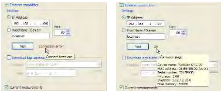
Figure 4.2. Example of network settings for a device that does not exist in the network (on the left) and correctly configured (on the right)
